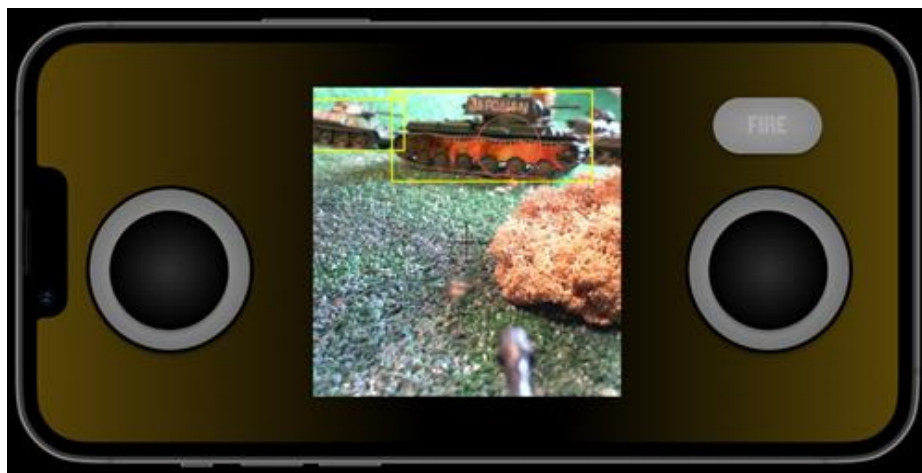
Figure 50: UI Mock-Up of Photo-TANKS Controller application's "Main Controller Interface" screen with firing systems disabled
