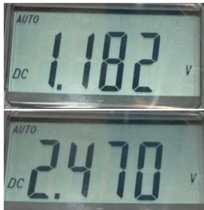
Figure 64: Voltage Across First Resistor, Low Power (top), High Power (bottom)
