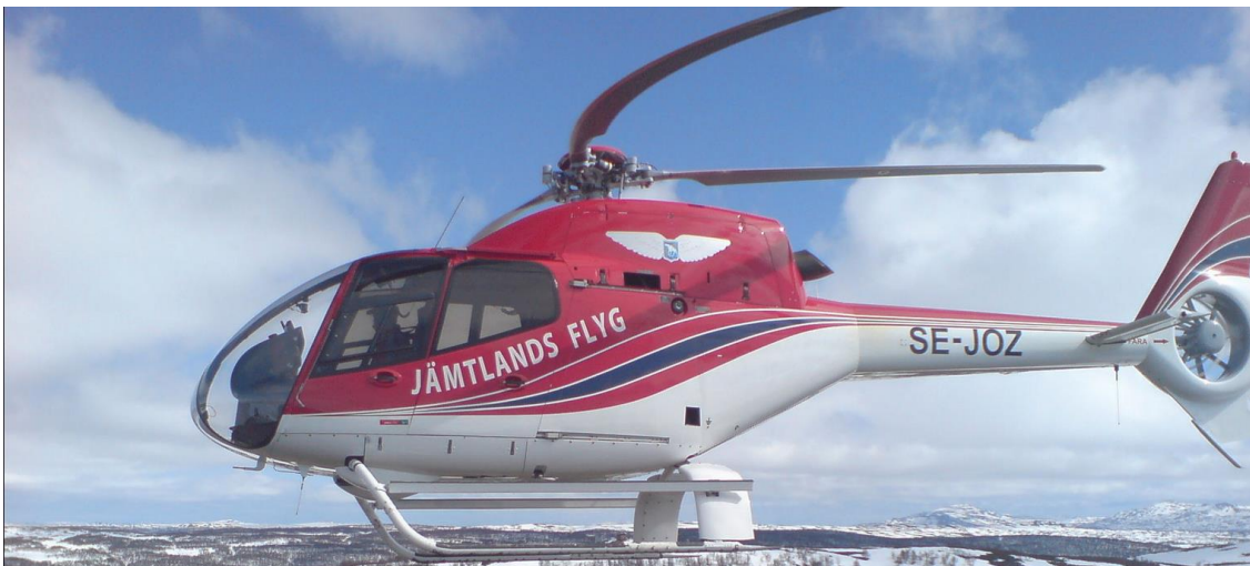
Figure 29: Rolling Shutter Distortion
